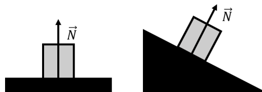
Figure 68: The normal force, \vec{N} , exerted by a horizontal surface on a block (left side) and by an inclined surface (right side). In both cases, the normal force on the object is perpendicular to the interface between the object and the surface and points in the direction from the interface towards the object.
